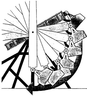
**Propped counterweights** allowed engineers to squeeze even more energy out of the counterweight. By propping up the counterweight at an angle before firing, they gave it slightly farther to fall. This innovation also increased the distance between the center of gravity of the counterweight and the pivot around which the trebuchet beam rotated.
